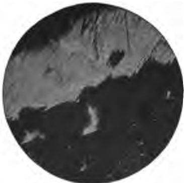
Fig. 31. Casehardened Steel showing Unequal Carburization
